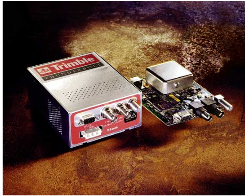
Trimble's Thunderbolt GPS Disciplined Clock in enclosure, and board form.
